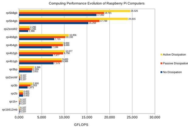
Fig. 1. Computing performance of Raspberry Pi computers over time
