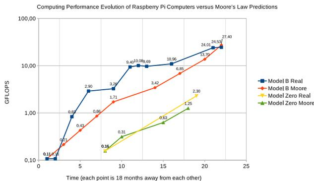
Fig. 3. Performance gain between Raspberry Pi generations versus Moore's Law.
