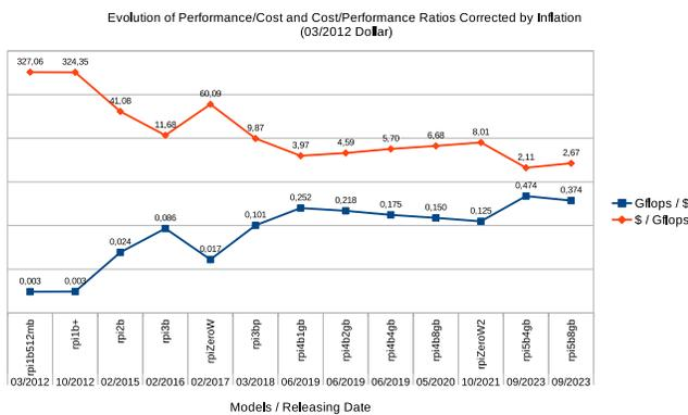
Fig. 2. Evolution of cost/performance ratio of Raspberry Pi computers
