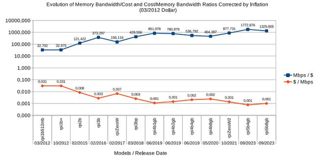
Fig. 7. Evolution of Memory Bandwidth/Cost ratio on Raspberry Pi computers
