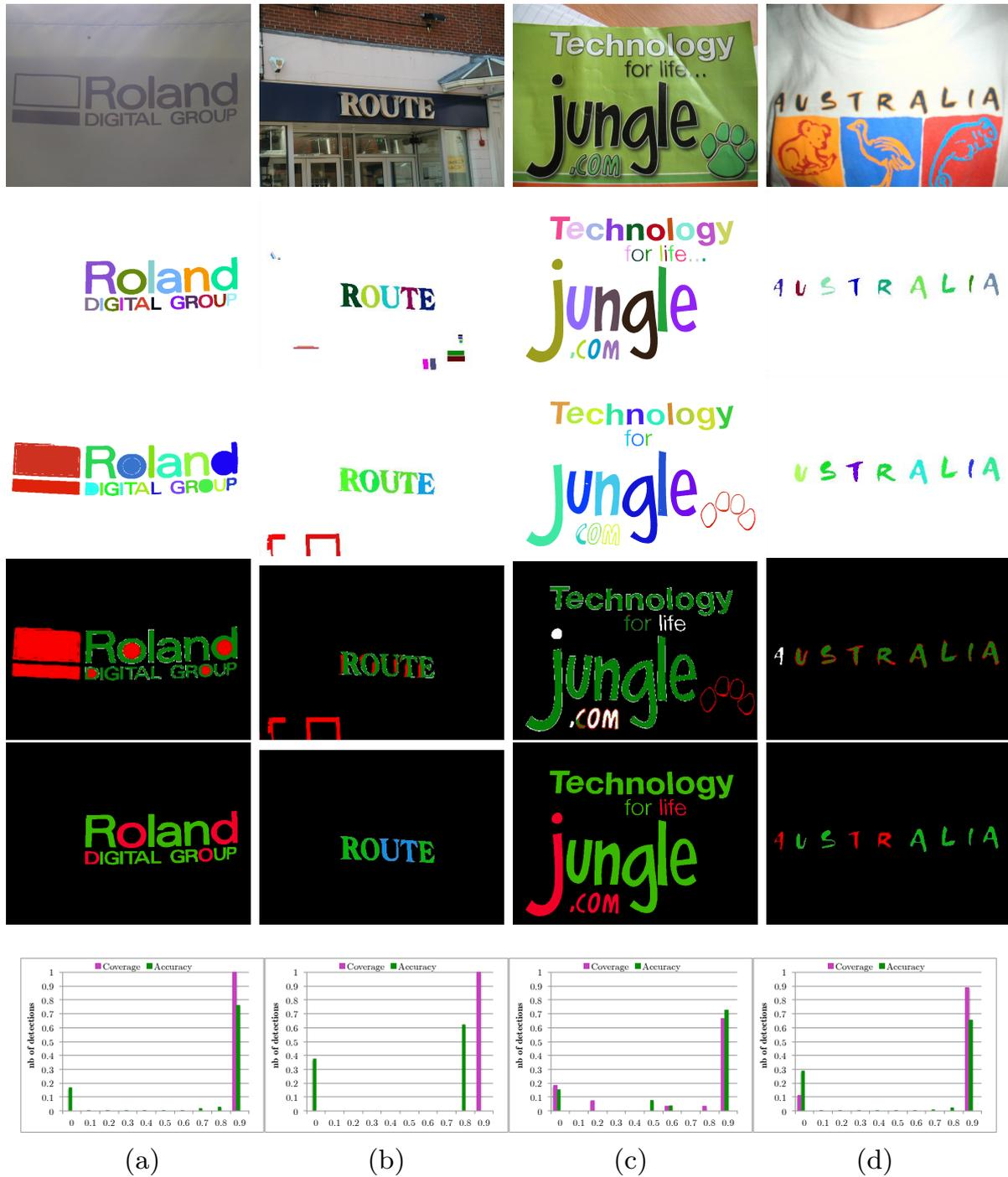
Fig. 2: Four examples (a, b, c and d). For each example, from top to bottom: the original image, the GT, the segmentation, the pixel-based classification (false positive in red, correct in green, non-segmented in white), the atom-based classification (non-detected in red, correct in green, merged in blue) and the histogram visualization.
