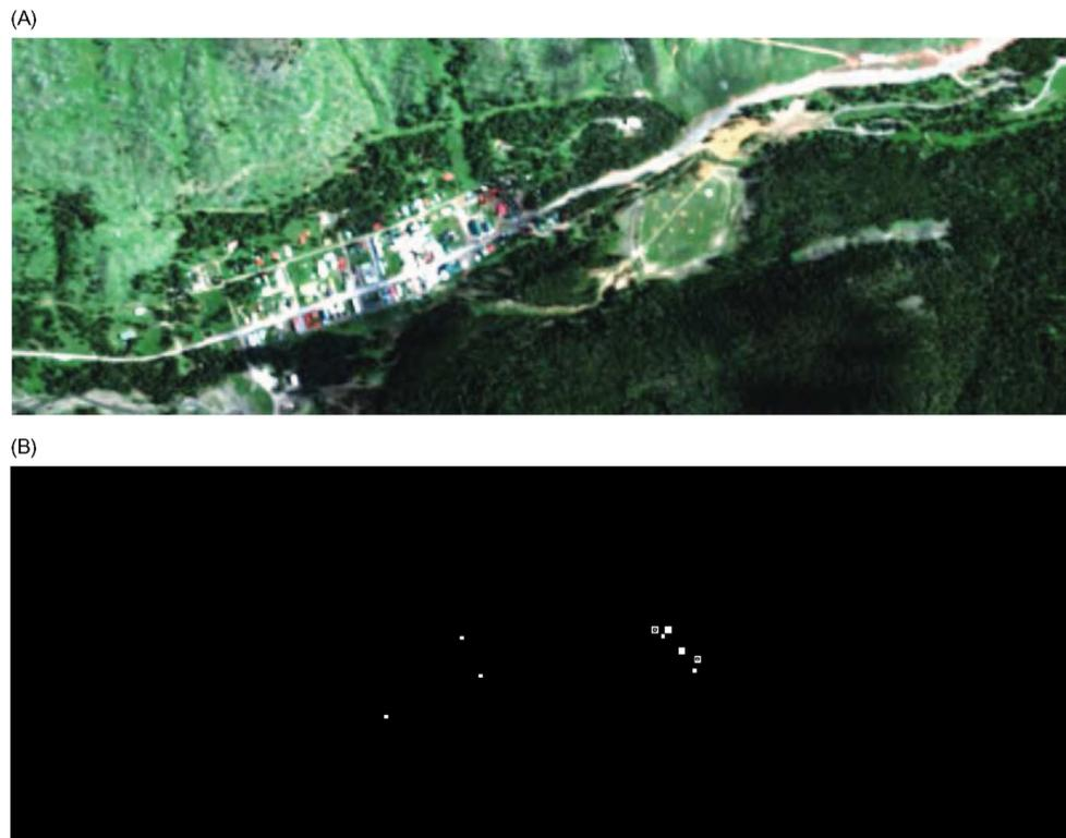
**Fig. 15** (A) False color representation of the Target Detection Blind Test hyperspectral data set, and (B) location of the targets in the scene.
