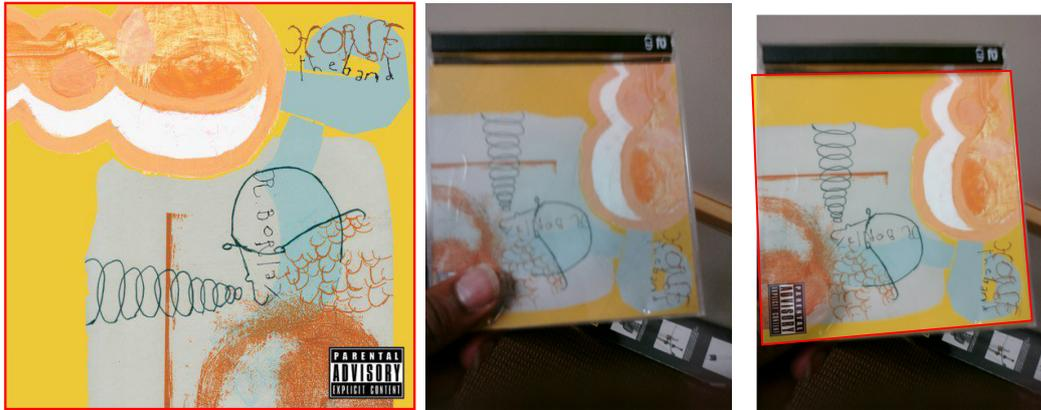
Figure 4.11: Homographic registration of a pair of images. Left: reference image. Middle: target image. Right: registration result using TBMR. All the other tested detectors using standard parameters do not provide a correct registration.
