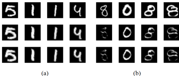
Fig. 11. The results of learning grayscale (a) dilation and (b) erosion operations by MNN. The first row shows the original images, the second row shows the target images, and the third row shows the output of the network after training 20 epochs.
