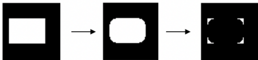
Fig. 4. The morphological residual model. Applying opening on the original image with circle structuring elements, then subtraction of result image from original image can obtain the morphological residuals.
