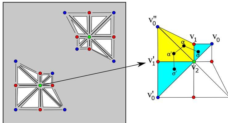
**Fig. 5.** How to compute the path joining two cells,  $\sigma := \langle v_0, v_1, v_2 \rangle$  and  $\sigma' := \langle v'_0, v'_1, v_2 \rangle$ , both incident to  $\langle v_2 \rangle$ . Since we are in the case  $i \neq i'$ , we compute two new cells  $\alpha$  and  $\alpha'$  which “join”  $\sigma$  and  $\sigma'$ : the final path joining  $\sigma$  and  $\sigma'$  is  $\pi = \langle \sigma, \alpha, \alpha', \sigma' \rangle$ .
