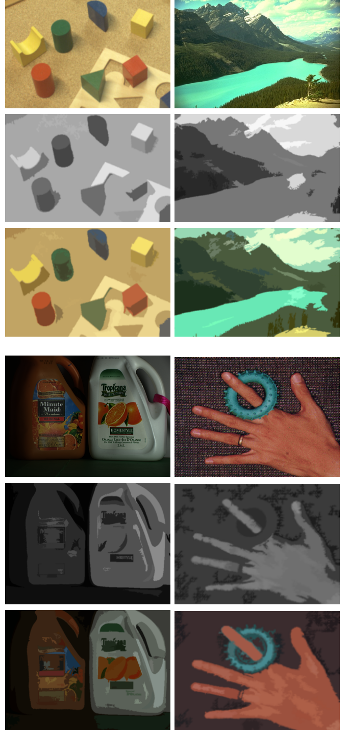
Fig. 7. Results of simplification. First row: original images. Second row: simplification by thresholding the saliency map of the tree of shapes on luminance. Third row: simplification by thresholding (with the same value) the saliency map of the tree of shapes on colors.
