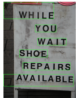
(f) Oversized detection can disturb EPs: IOU/DE/I13 validate the word “Available” but not “while”.
