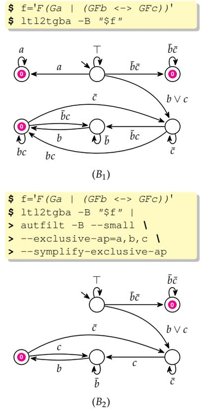
Figure 2.15: Automata for  $\varphi = F(Ga \vee (GFb \leftrightarrow GFc))$ . Automaton  $B_2$  is a simplified version of  $B_1$  assuming that  $a, b$  and  $c$  are mutually exclusive.
