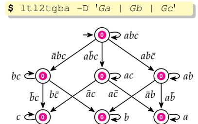
Figure 2.11: Top: non-deterministic BA for  $G_a \vee G_b \vee G_c$ . Bottom: minimal equivalent WDBA.
