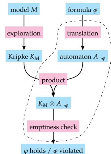
Figure 1.1: The automata-theoretic approach to LTL model checking. The dashed curve shows the parts we focus on.
