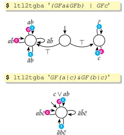
**Figure 5.2:** The translation offered for  $(GFa \wedge GFb) \vee GFc$  is inferior to that given for the equivalent formula  $GF(a \vee c) \wedge GF(b \vee c)$ .
