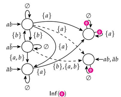
**Figure 6.9:** A 1-pass testing automaton can be obtained by using non-determinism (dashed lines) to capture stuttering runs into a dedicated state.
