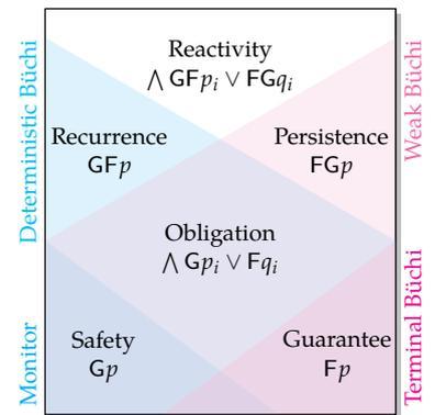
**Figure 2.4:** The temporal hierarchy of Manna and Pnueli [1990], labeled by canonical LTL properties where  $p$  can be any subformula that uses only Boolean operators,  $X$ , or past LTL operators. Any persistence property (this includes the obligation, safety, and guarantee subclasses) can be represented by a weak Büchi automaton and cannot benefit from transition-based Büchi acceptance.
