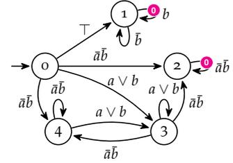
Figure 2.17: An unambiguous BA for  $GFa \rightarrow GFb$ . Here the word  $\bar{a}b; \bar{a}b; \bar{a}b; \dots$  has a unique accepting run.
