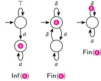
Figure 4.3: Three minimal automata for  $\text{FG}a$ , using: state-based Büchi acceptance, state-based co-Büchi acceptance, and transition-based co-Büchi acceptance.
