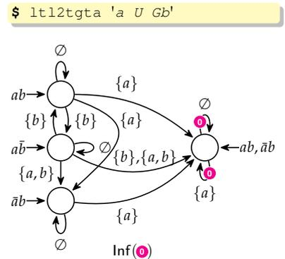
Figure 6.10: A Transition-based Generalized Testing Automaton for  $a U Gb$ . Here the acceptance condition use a single Büchi set, but it could use more.
