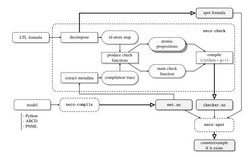
Fig. 1. The architecture of Neco.
