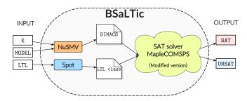
Fig. 2: BSaLTic's Framework. The dashed box represents the BSaLTic tool
