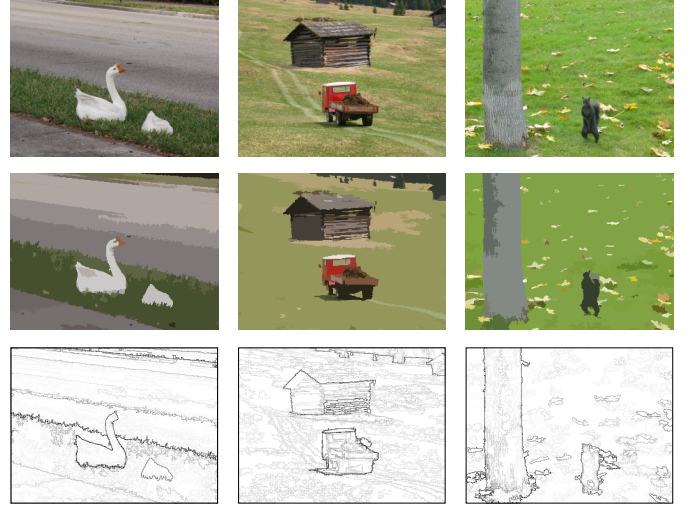
Fig. 7: Some pre-segmentation results obtained with our proposed method on the segmentation evaluation database in Alpert et al. (2012). Top: input images; Middle: pre-segmentations obtained with the simplification method; Bottom: inverted saliency maps for hierarchical simplifications.
