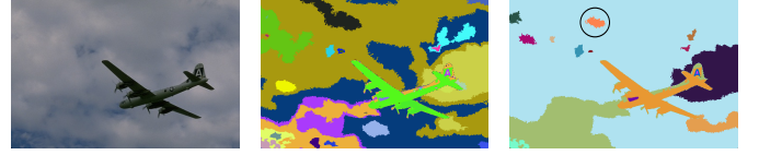
Fig. 4: Illustration of causality principle violation. Left: input image; Middle and right: randomly colored simplified image with \lambda_{s1} = 100 and respectively \lambda_{s2} = 500 . The orange shape on top middle of the right image (surrounded by a black circle) is preserved for \lambda_{s2} = 500 , while it is removed for \lambda_{s1} = 100 in the middle image.
