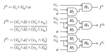
**Fig. 19**: Encoding of functions  $f^x$ ,  $f^{\ell_0}$ ,  $f^{\ell_1}$  as And-Inverter Graphs based on Irredundant Sums-of-Products.
