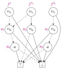
**Fig. 16**: BDD representation of  $f^x$ ,  $f^{\ell_0}$ , and  $f^{\ell_1}$  from Figure 15. A BDD is like a decision tree with sharing of identical subtrees. Each round node is labeled by a Boolean variable that is questioned, plain edges should be followed when the variable is true, and dashed edges when it is false. Variables always appear in the same order along a branch.
