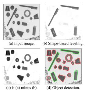
Figure 3. Illustration of shape-based leveling and object detection.
