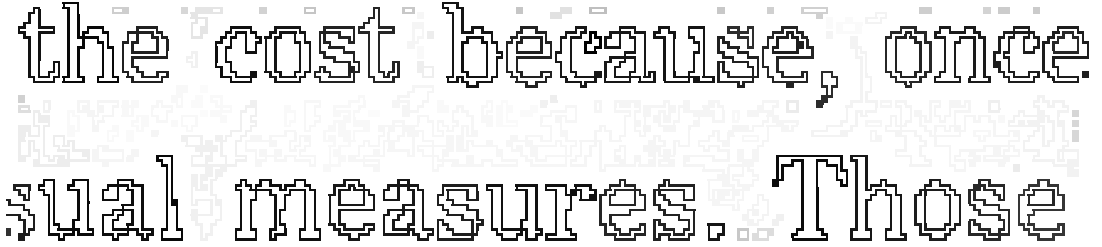
Figure 5.: Zero-crossings of the original Laplacian
