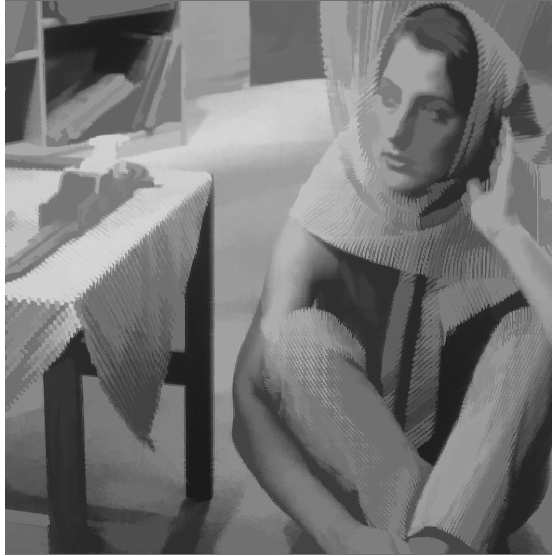
Figure 10.: A grain filter of the DWC interpolation of the Barbara image with a threshold \lambda = 1280
