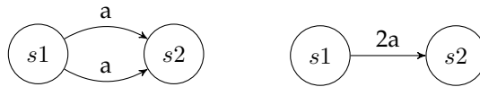
Figure 4.7: Multiple label issues. The left automaton is wrong, the one on the right is the expected \mathbb{Z} -automaton.
