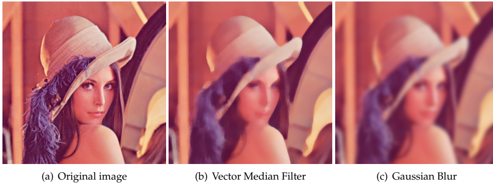
Figure 3.1: Comparative of denoising filters. Size of window is 9x9.
