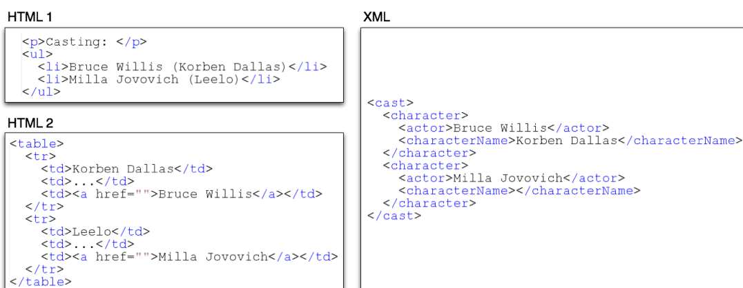
Figure 6.1: Example of XML heterogeneity. The same movie description extracted from three sources: two HTML styles and one XML general movie schema.
