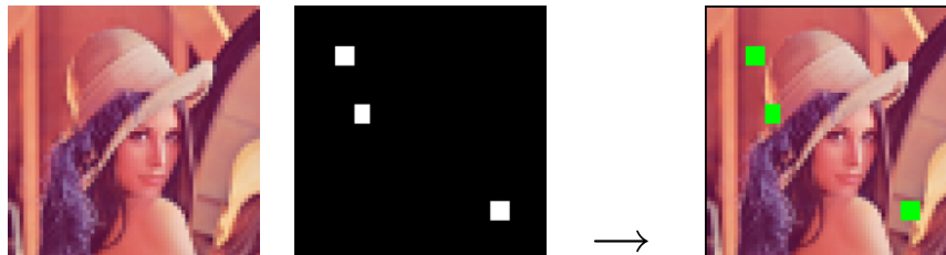
Fill with green a region of interest defined by a mask image.
