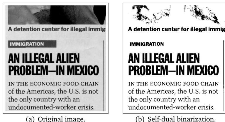
Figure 2.12 – Text segmentation with our method can be seen as a binarization technique, providing also reverse-video text.
