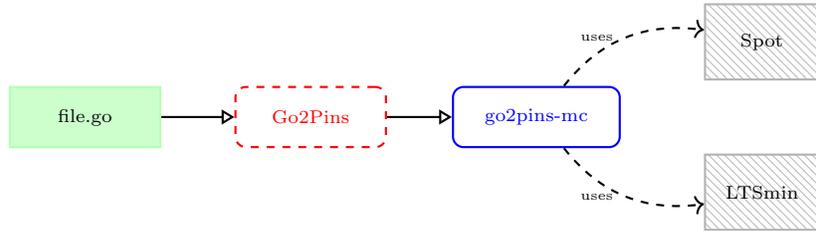
**Fig. 1.** Overview of Go2Pins. The input file is processed by Go2Pins which produces a binary called **go2pins-mc**. This binary can then be used to verify LTL formula using one of the two supported backends: Spot or LTSmin.
