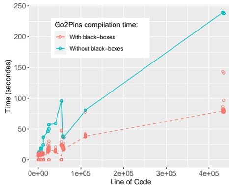
**Fig. 3.** Time required by Go2Pins to process and compile an input go program according to its number of line of code. Dots represent one computation in the benchmark (a pair model-formula), while lines join the mean of each series.
