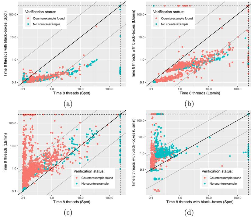
**Fig. 4.** Time comparison in  $\log_{10}$  scale for each backend (Spot and LTSmin), with or without black-boxes. The dark line corresponds to identity while gray lines show the 10 factor speedup/slowdown. Dashed lines represent the 4 minutes timeout.
