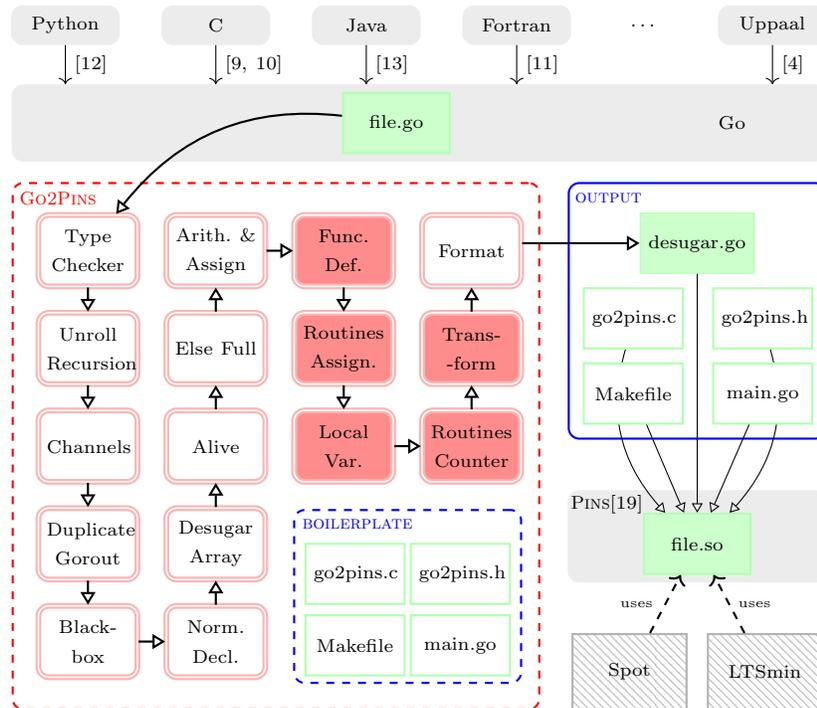
**Fig. 2.** Contributions of this paper (all except gray boxes). The dashed boxes represent the Go2Pins tool while the blue plain box represents the output directory produced by Go2Pins. The transformation steps are denoted by double shaped red boxes. Files grouped under the name *boilerplate* are copied as-is into the output directory. These files are generic and handle communication between the desugared program and the mandatory functions to respect the PINS interface.
