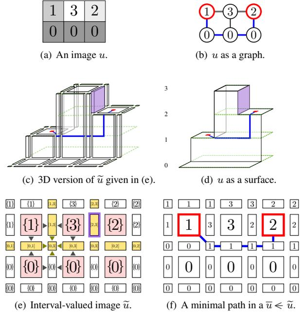
Fig. 1. Image representations for computing barrier distances.
