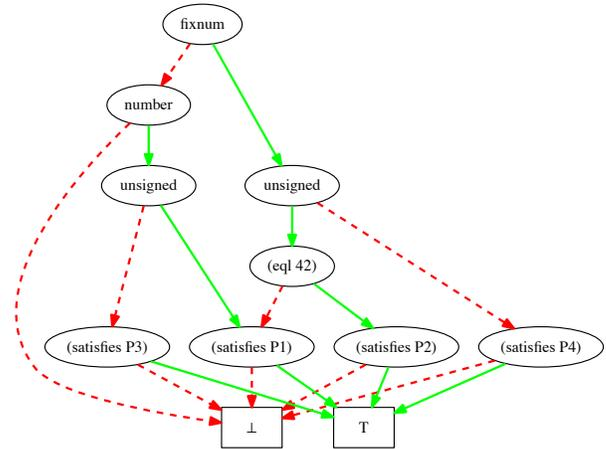
Figure 9: ROBDD from `typecase` clauses in Example 7
