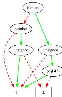
Figure 6: Common Lisp type, `(or (not number) (eql 42) (and fixnum (not unsigned)) (and unsigned (not fixnum)))` represented as ROBDD. The symbols  $\perp$  and  $\top$  refer to *false* and *true* respectively.
