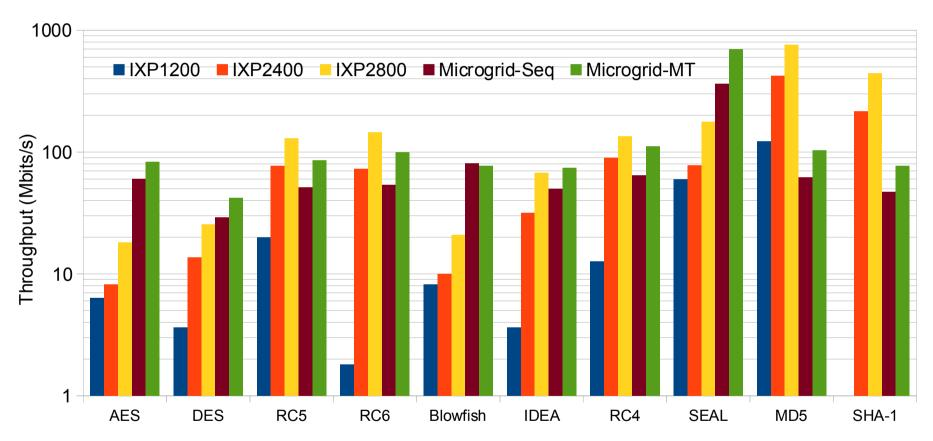
Intel IXP = embedded processor specialized for cryptographic workloads
