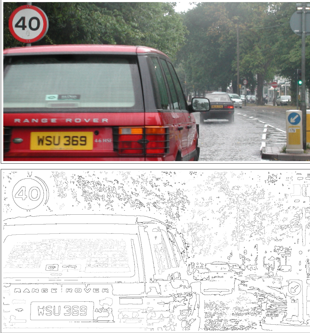
Figure B.1: Hierarchical representation of an image: since component boundaries are simple closed curves on well-composed images, two boundaries are either disjoint or in an inclusion relationship; thus, the delimited regions naturally form a tree. Actually it is a sub-part of the tree of shapes [60].
