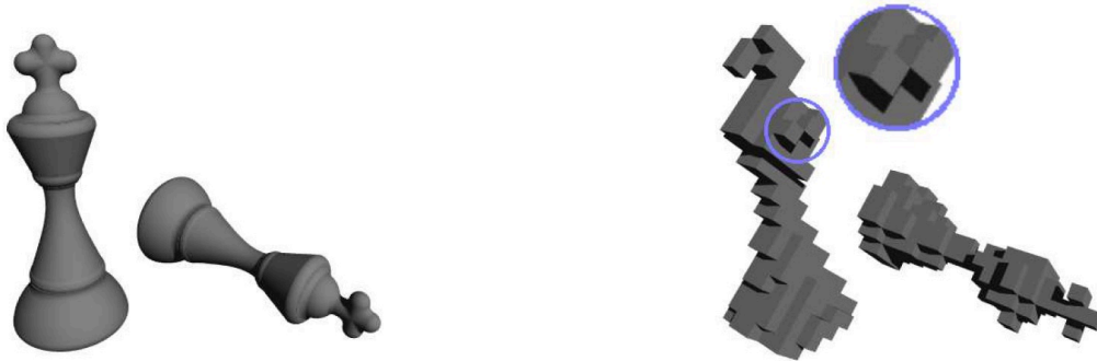
Figure 2.27: A reconstruction based on cubical grids in 3D leads to critical configurations [163].
