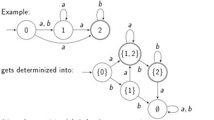
(Here the transition labeled a, b use syntactic sugar to represent two transitions a and b.)
