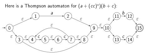
You can see in the construction rules that we always add two states (new initial and final states) each time we process a letter,  $\varepsilon$ ,  $\emptyset$ , or the operations + and \*. The only case we do not add states is in the concatenation operation.
