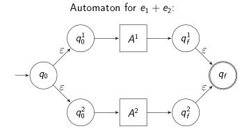
Here  $q_0^i$ ,  $A^i$ , and  $q_f^i$ , represents the automaton that has been recursively constructed for the regular expression  $e_i$ .  $q_0^i$  and  $q_f^i$  are the designated initial and final states, while  $A^i$  denotes the rest of the automata.
