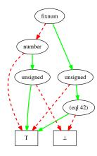
Figure 6: Common Lisp type, (or (not number) (eq1 42) (and fixnum (not unsigned)) (and unsigned (not fixnum))) represented as ROBDD. The symbols  $\perp$  and  $\top$  refer to *false* and *true* respectively.
