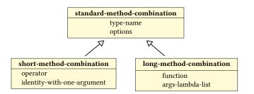
Figure 2: SBCL Method Combination Classes Hierarchy
