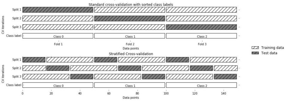
Stratified: Ensure relative class frequencies in each fold reflect relative class frequencies on the whole dataset.
