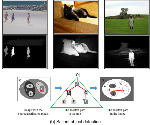
Fig. 1: Image processing with the max-tree. (a) Background extraction for document image analysis with a morphological black top-hat. The min-tree is pruned by removing connected small peak components ( < 4 pixels that do not touch the border). The residue (filtered components) forms the clean text and the background is removed. (b) Saliency object detection for scene analysis [1]. A morphological tree is used to compute the Dahu distance from image borders. This distance that mixes geodesic distance and gray-level distances can be computed using a tree similar to the max-tree (the tree of shapes).
