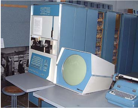
First minicomputer: the PDP-1
