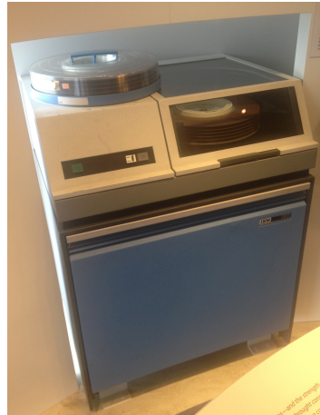
Removable disks on IBM 1311 (6 disks, 2.6MB)
